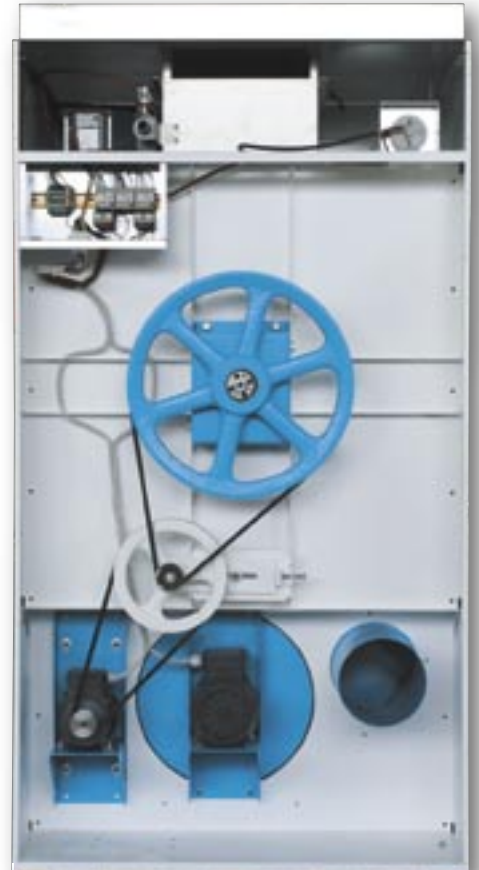
Reversing drum is standard on models ES 23-34-55
