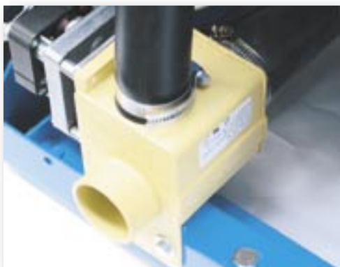
The motorized drain valve can be fully opened allowing a direct flow of water avoiding any residual remaining
